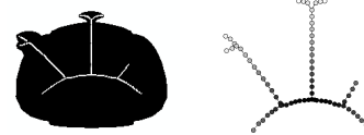
Figure 3. Left: the silhouette and its medial axis. Right: the medial axis tree constructed from the medial axis. Darker nodes reflect larger radii.
