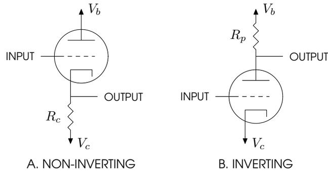
Figure 2. Triode Switching Circuits
