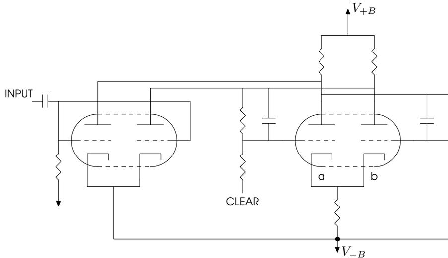
Figure 10. PM Flip-Flop
