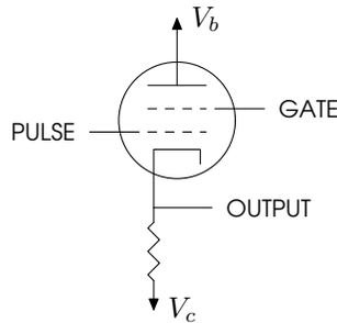
Figure 3. Tetrode Gate (AND) Circuit
