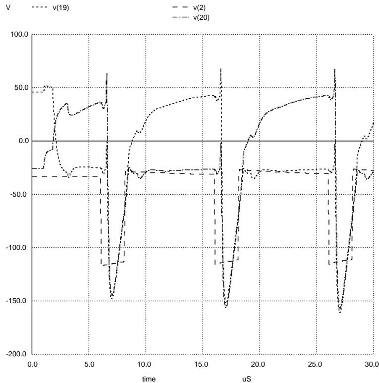
Figure 11. SPICE Simulation of PM Flip-Flop
