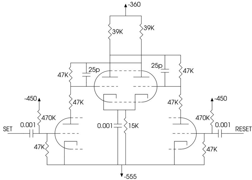
Figure 6. Typical Flip-Flop Usage
