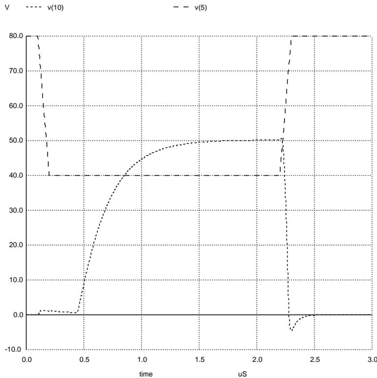
Figure 15. SPICE Simulation of Transmitter
