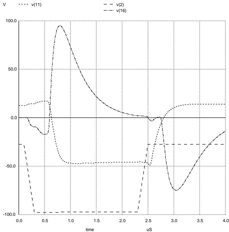
Figure 13. SPICE Simulation of Pulse Standardizer
