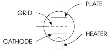
Figure 1. Triode Schematic Symbol
