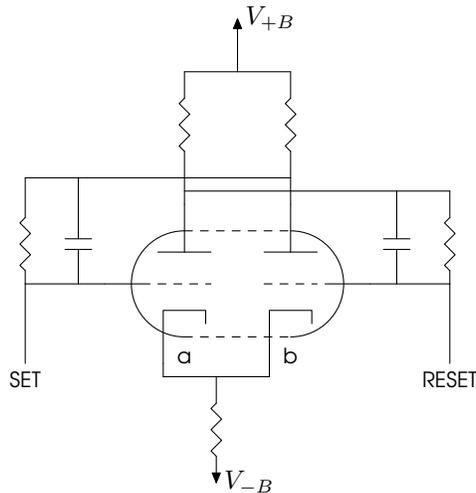
Figure 5. Basic Flip-Flop Circuit
