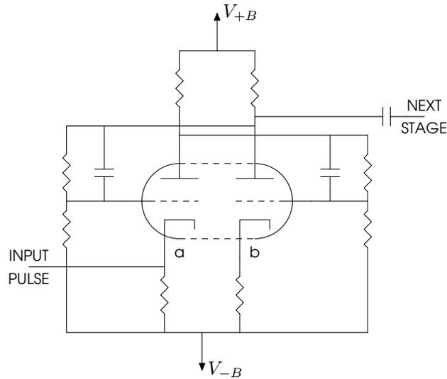
Figure 8. Flip-Flop Used in Multi-Stage Counters
