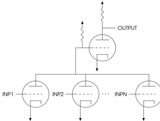
Figure 4. Direct Coupled OR Circuit
