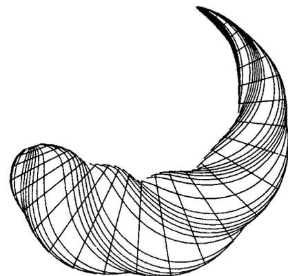
Figure 2.4.4 a Bent, Twisted, Tapered Primitive
