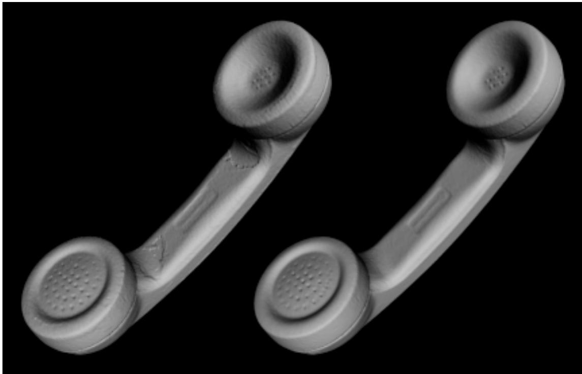
**Figure 9:** Left: This model of a telephone handset was created by zippering together meshes from ten range images. The mesh consists of more than 160,000 triangles. Right: The final positions of the vertices in the mesh have been moved to an average of nearby positions in the original range images. We call this the consensus geometry.
