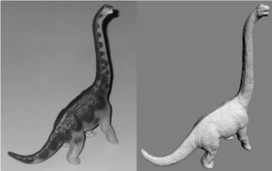
**Figure 8:** Photograph of a plastic dinosaur model (left) and a polygon mesh created by registering and zippering together 14 range images that were taken of the model (right). The mesh consists of more than 360,000 polygons.
