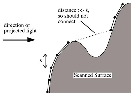
**Figure 3:** Building triangle mesh from range points.
