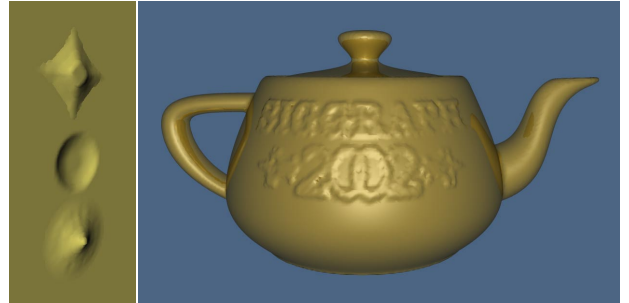
Figure 8: Left: Three types of single point attractions/repulsions using different ROI primitives and \gamma values. Right: Utah teapot embossed with 7862 points sampling the “SIGGRAPH 2002” logo.
