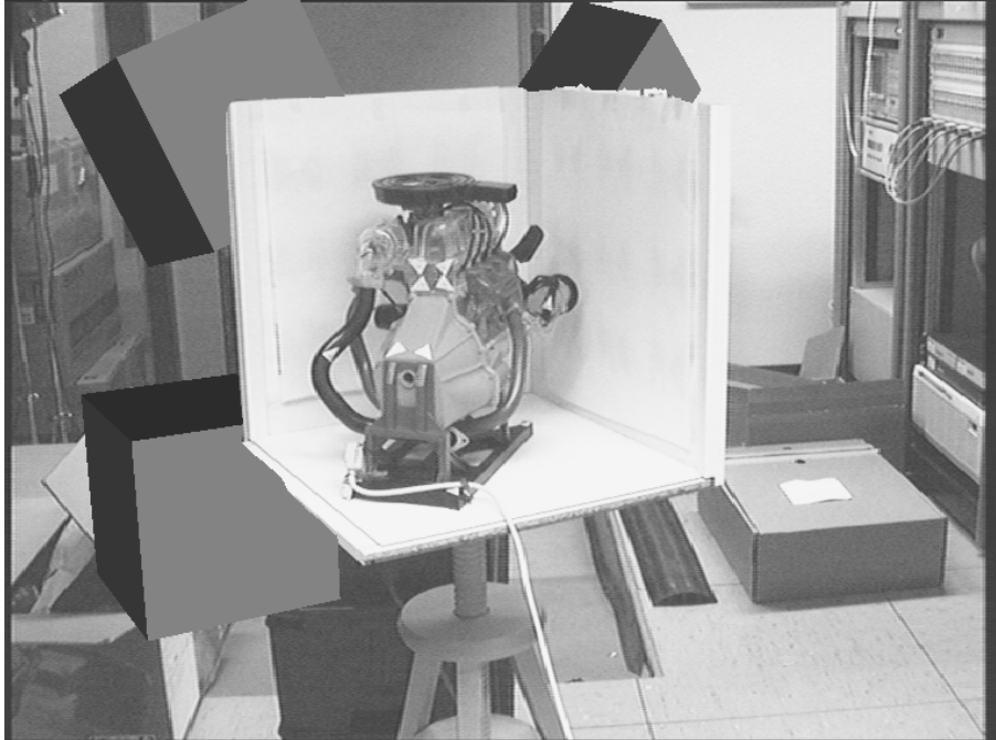
Figure 6: Three virtual cubes occluded by a wooden stand and occluding the room background, using the depth-based technique.
