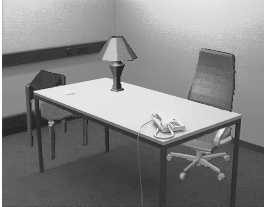
Figure 5: A real table occludes two virtual chairs in augmented reality, while being occluded by a virtual lamp, using the model-based technique.
