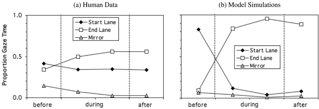
Figure 6. Lane-changing profiles for proportion gaze time on the start lane, end lane, and mirror for (a) human data and (b) model data. The vertical dotted lines indicate the start (leftmost line) and end (rightmost line) of the lane change.
