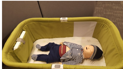
Figure 1: The Bellyband can be seen here worn around the Laerdal SimBaby’s waist. There are no wired connections or additional nodes required for its function. As the torso expands upon inhalation, the band will stretch, causing changes in the Received Signal Strength Indicator (RSSI), which we then use to infer breathing patterns.
