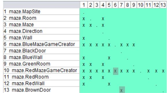
Figure 3: The Maze DSM prior to applying *Split* operator. All variables form a single large module, and the highlighted dependencies are candidates for introducing new design rules.
